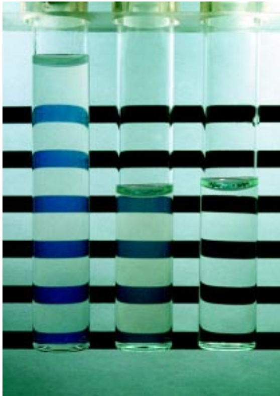
Figure 9-3. Comparison of McFarland 0.5 with inoculum suspension. From left to right, the tubes are the McFarland 0.5 standard, E. coli ATCC 25922 adjusted to the 0.5 McFarland turbidity, and uninoculated saline.
